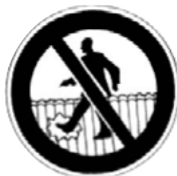
Figure 6: Warning sign to be used on brittle and fragile roofs
