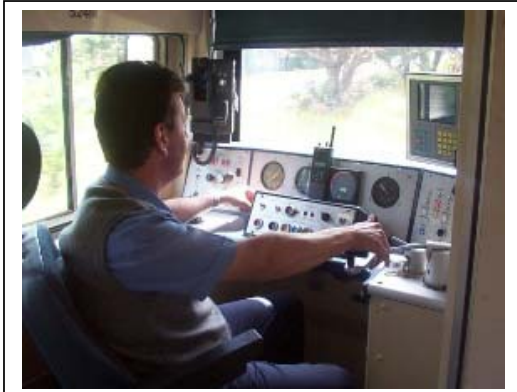
Driver in cab - right hand on power/deadman's handle.
