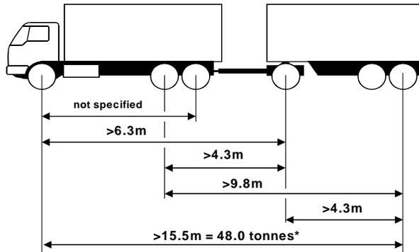
\* For a 48 tonne load, the extreme axle spacing must be more than 15.5 metres. Reduce the total load of the combination by 0.5 tonnes for each 0.5m reduction in extreme axle spacing.
