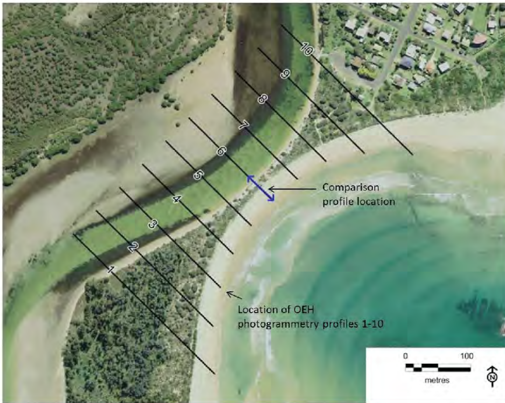
Figure 12: Location of OEH photogrammetry profiles and 2014 comparison profile
