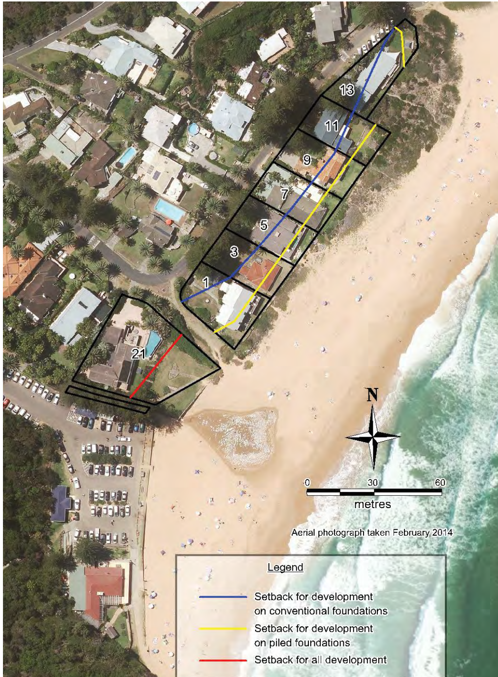
Figure 22: Adopted minimum beachfront setback lines for development on conventional and piled foundations at Bilgola Beach
