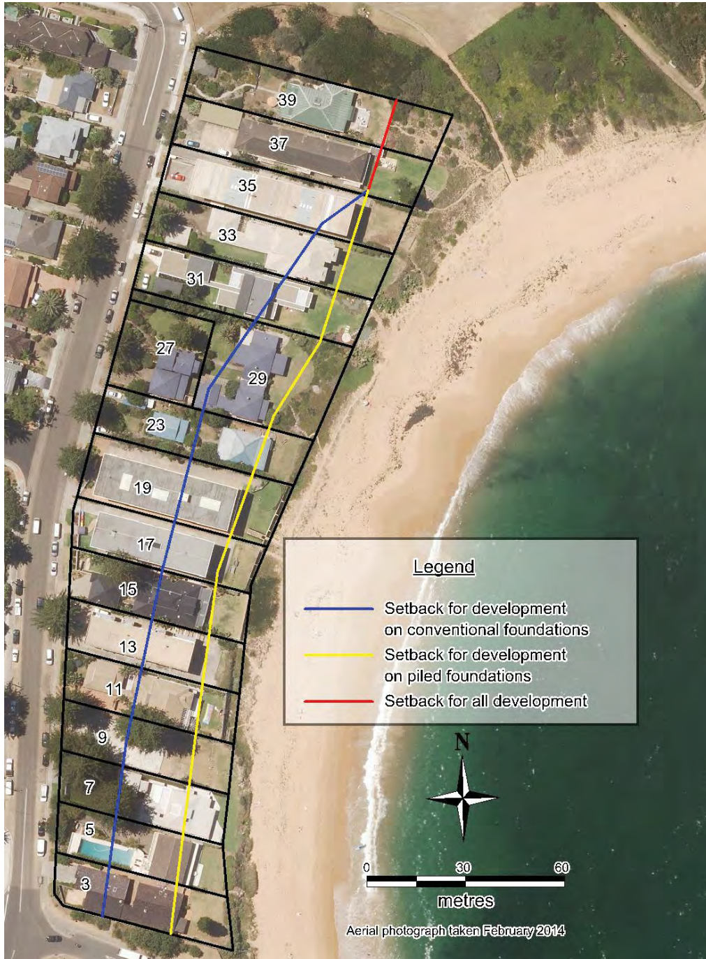
Figure 23: Adopted minimum beachfront setback lines for development on conventional and piled foundations at Basin Beach
