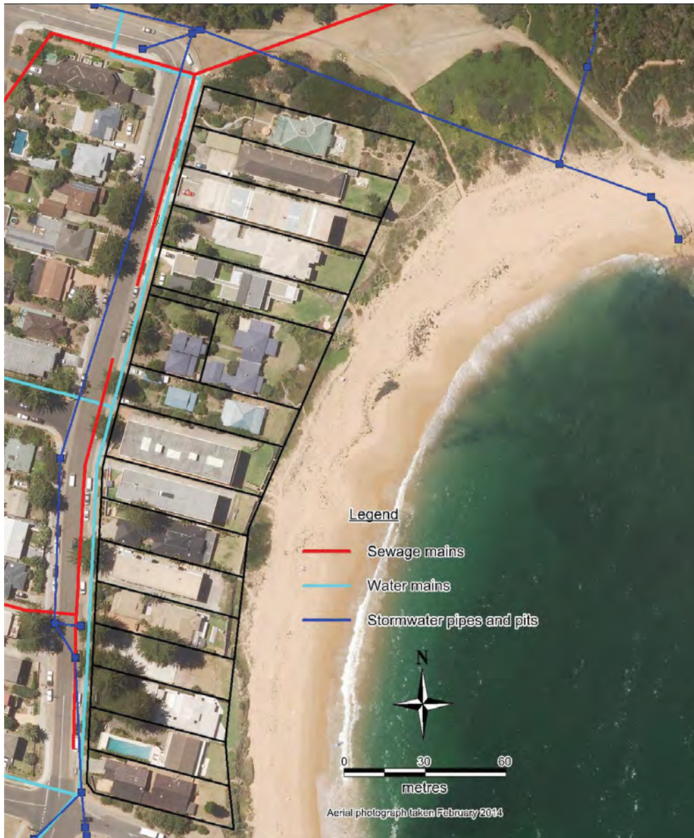
Figure 9: Stormwater, sewage and water infrastructure locations at Basin Beach
