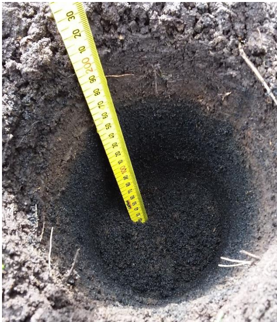
Annexure B – Metallurgical slag on soil surface (top), as in-fill below topsoil (bottom left) and zoomed metallurgical slag on soil surface impacted soil (bottom right)
