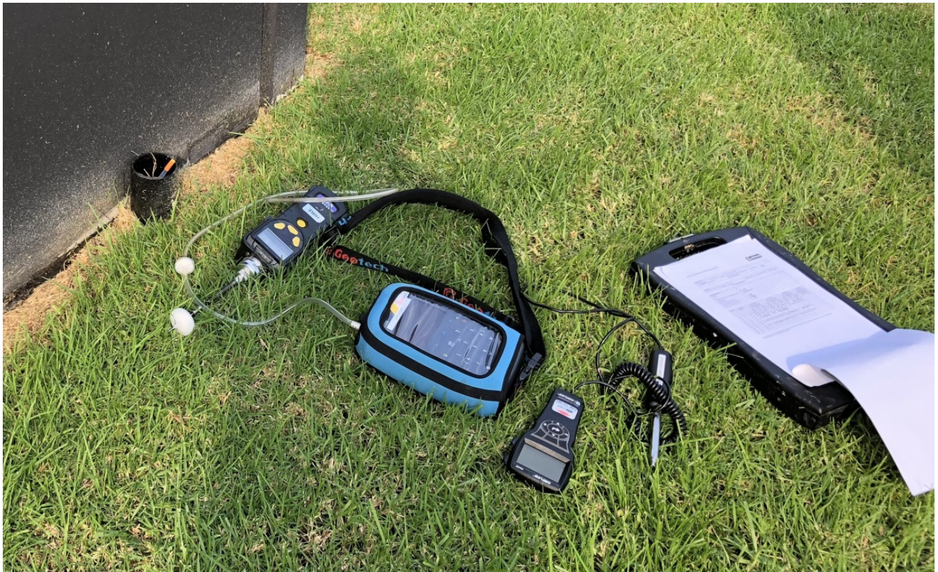
Figure 20 GA5000, MiniRae and Velocicalc in use for subslab and riser measurements
