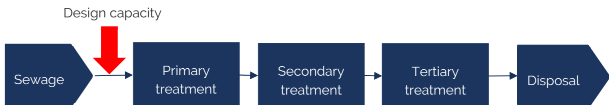
Figure 2.3 An example diagram showing where design capacity should be determined for treating sewage for disposal only
